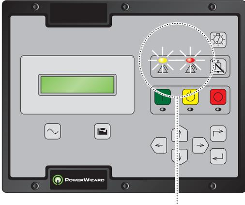
If either of these indication lamps are flashing or solid there is a warning or shutdown
